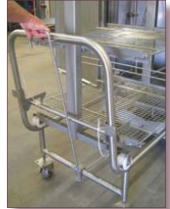
Cart docks and locks to cabinet rails. Rack is released to roll easily into washer.
