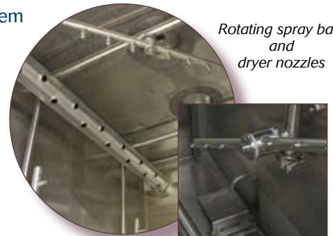
Quick disconnect on spray bars allows easy access and inspection
