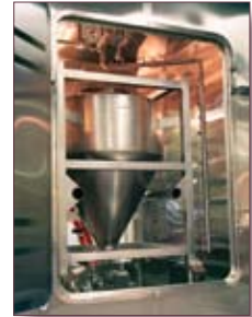
IBC Tote with cover removed for cleaning
